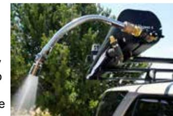
**Spray Nozzle:** The spray nozzle can be adjusted to a variety of spray patterns. Just rotate the tip of the nozzle to adjust the shower spray to jet setting. If the tip is completely tight, no water will come out. You can also remove the nozzle and run the water from the hose alone. Be sure to attach the nozzle prior to travel by using the hose clip and Velcro.
