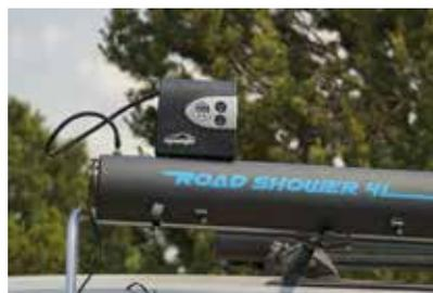
**!** This product releases pressure at a target of 65 PSI. If the pressure relief valve on the fill cap is damaged or is altered, the Road Shower could explode and cause injury and possibly death. Check pressure while pumping air and never pressurize greater than 75 PSI. If the pressure is not releasing before it reaches 75 PSI, the fill cap should be replaced.
